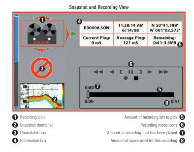
**NOTE:** For snapshots and recordings, the indicator bar has several states: during recording, the amount of space remaining on the SD card is indicated on the status bar. During playback, the amount of time/memory remaining to play is indicated on the status bar. When a snapshot thumbnail is highlighted, the amount of room remaining on the SD card is indicated.
